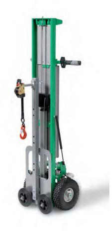
Max. liftcapacity: 75 kg Liftingspeed: 100 mm/s Max. liftingheight: 1.10 m
